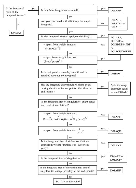
\*D01ATF and D01AUF are likely to be more efficient than D01AJF and D01AKF, which use a more conventional user-interface, consistent with other routines in the chapter.
